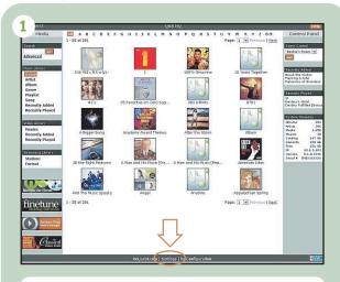
Connect to the web server of the ReQuest server by entering the server's IP address in a web browser. Click "Settings" on the bottom.
